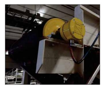
Equipment manufacturers and conveyor operators have used Rulmeca internally powered conveyor belt drives throughout the world, since their introduction in the 1950s. They prefer the Motorized Pulley's compact size, light weight, reliability, safety, and ease of maintenance when compared with the limitations of exposed drive systems.
