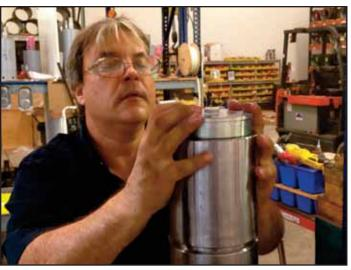
Rulmeca Motorized Pulley diameters of 4.45", 5.45", and 6.49" are most popular in unit handling and food processing applications. However, Rulmeca's complete portfolio includes eleven models, from the tiny 3.15" diameter 0.16 HP unit to the huge 40.16" diameter 330 HP monster. When combined in "multiple drive configuration", conveyor drive power is virtually unlimited.
